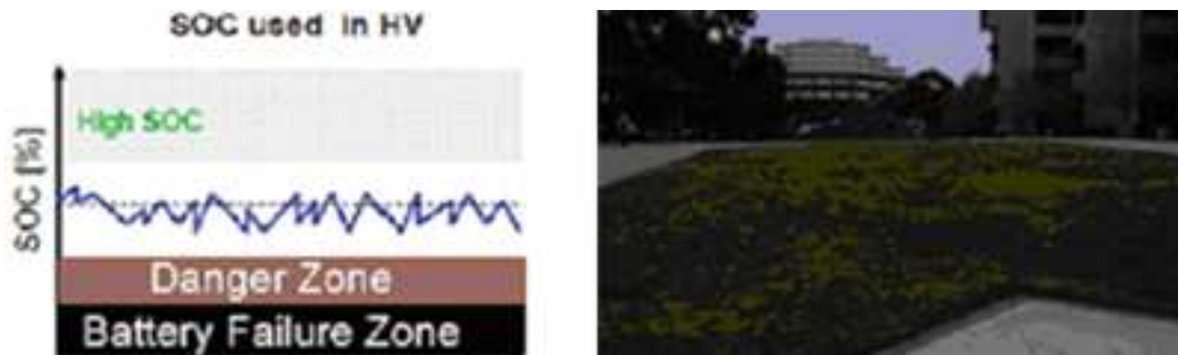
Figure 3 – Hybrid Vehicles have reliable long-lasting batteries because the system is designed to keep the batteries in the safe State-of-Charge area (Blue line). The green island in a convenient central park location, like above, can put batteries back into the safe zone for the return trip.
